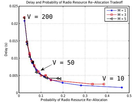
Fig. 6. Tradeoff between delay and probability of resource re-allocation with different  $M$ .
