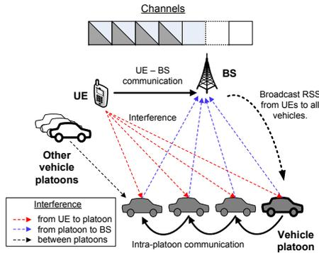
Fig. 1. Scenario: Vehicles drive in a platoon and communicate with each other underlying the UE-BS communication.
