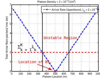
Fig. 3. There is no algorithm that can guarantee the delay of V2V communication underlying BS while the location of platoons is too close to the BS.
